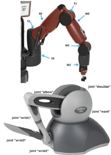
Fig. 3. Corresponding joints of Baxter (top) and the Geomagic Touch (bottom).
