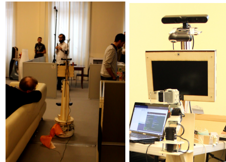
Fig. 11. RoCKIn Camp: a) Team demo b) Improved robot perception with a RGB-D camera on top of the platform
