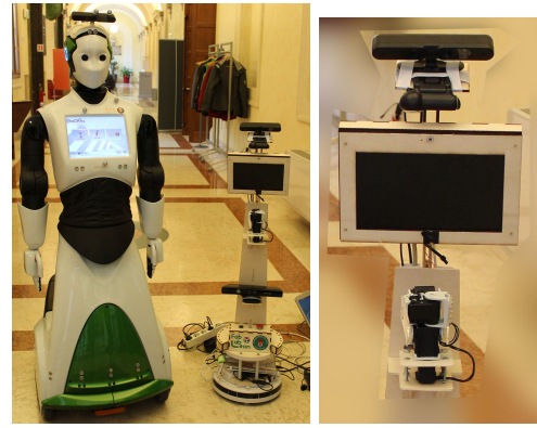
Fig. 9. a) REEM and MYRABot. b) Extra camera for object pose recognition
